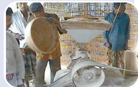
*Diesel powered rice mill project. Same motor that powers irrigation pumps.*
